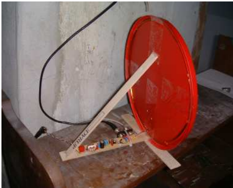
Figure 5. $20 homebrew loop antenna
