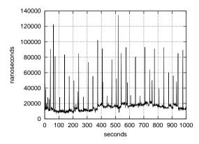
It is painfully obvious that the interrupt latency is the dominant noise factor in PPS timestamping in the second case. The asymetric distribution of the noise in the second plot also more or less entirely invalidates the design assumption in the NTP PLL/FLL kernel code that timestamps are dominated by gaussian noise with few spikes.
