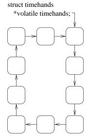
This scheme has an inherent risk that a process may be de-scheduled for so long time that it will not manage to complete the timestamping process before the entire ring of timehands have been recycled. This case is covered by each timehand having a private generation number which is temporarily set to zero during the periodic processing, to mark inconsistent data, and incremented to one more than the previous value when the update has finished and the timehands is again consistent.
